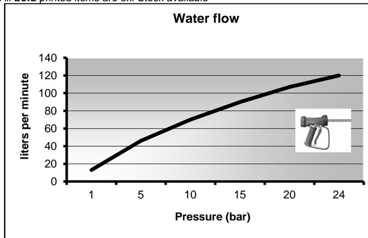
water flow in l/min with totally pulled trigger
